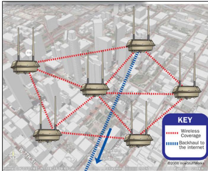
Figure 3. Conceptual Diagram of WiFi Mesh Network
