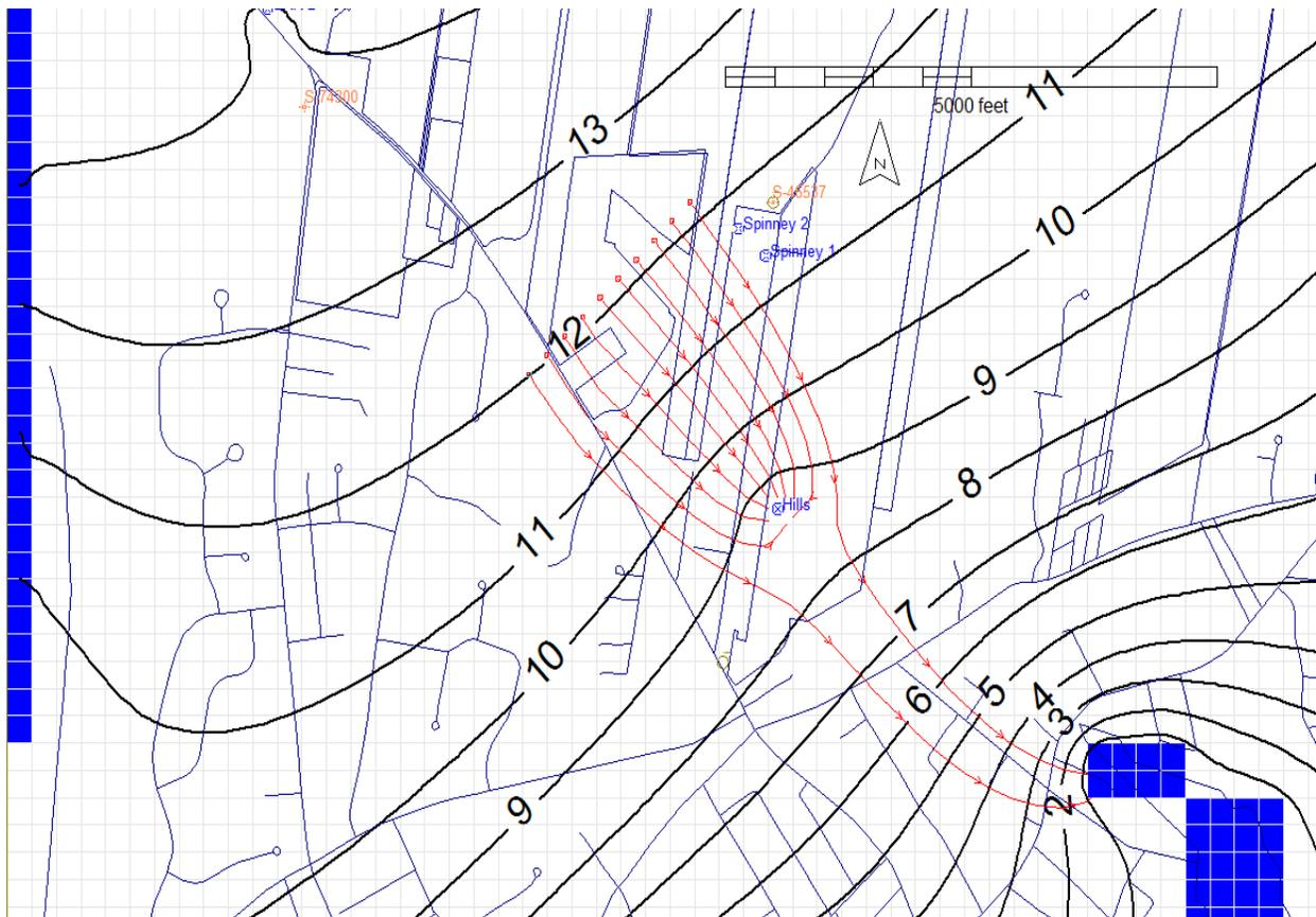
**Figure 3 – Hills Irrigation Well Location and Particle Tracks: Instantaneous Pumping Rate 300 gpm**
