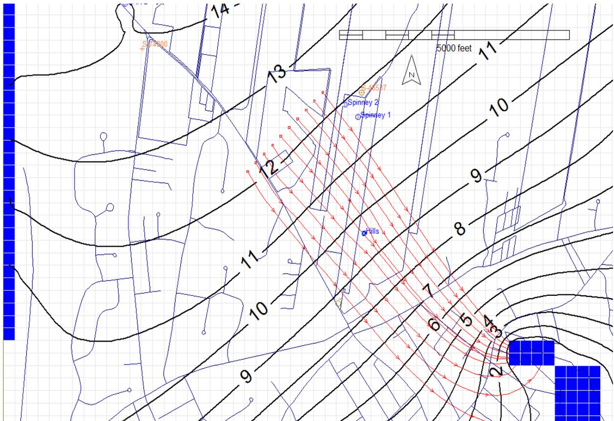
**Figure 3A - Hills Irrigation Well Location and Particle Tracks: Annualized Pumping Rate 38 gpm**
